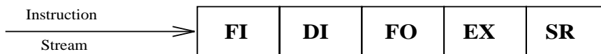
Figure 3: Pipelined execution of instructions. The steps are: FI, fetch instruction; DI, decode instruction; FO, fetch operand; EX execute instruction; SR store result. Since this pipeline has five segments, it can be operating on five instructions simultaneously. While the FI segment is fetching an instruction, the DI segment is decoding the previous instruction, and so on down the pipe.
